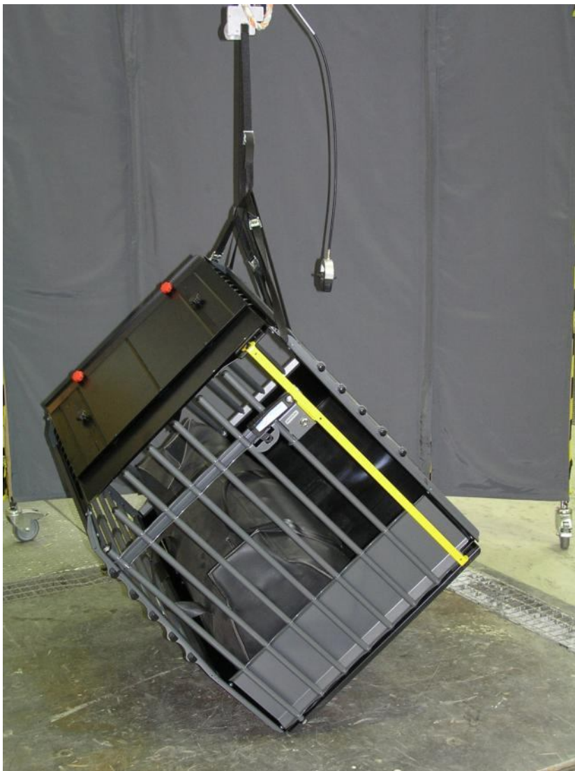
Figure 8, Angle adjustment of the test objects before the drop test
