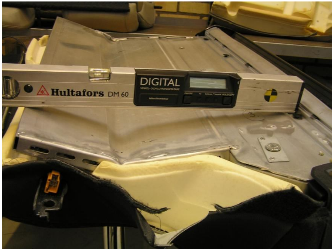
Figure 5, Measuring the horizontal deformation of the seat back
