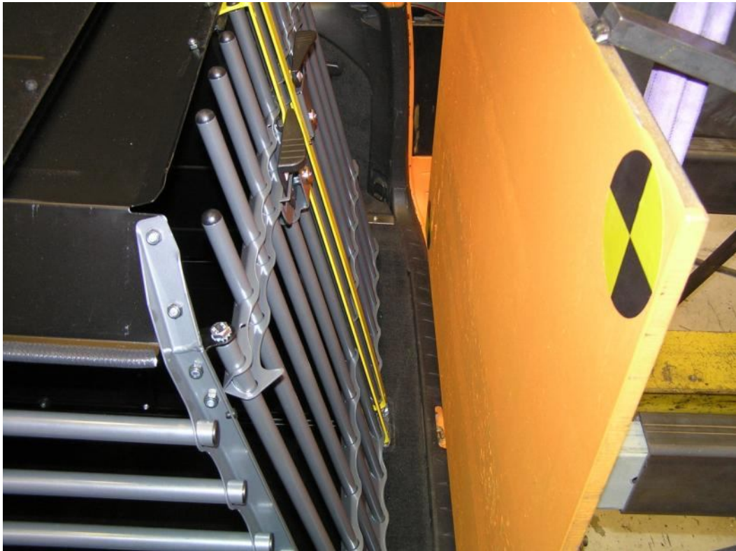
Figure 3, The crash barrier position when the crash bars starts deforming (braking)
