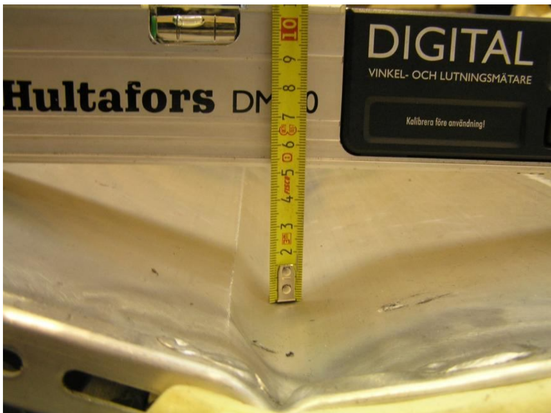
Figure 6, Measuring the horizontal deformation of the seat back
